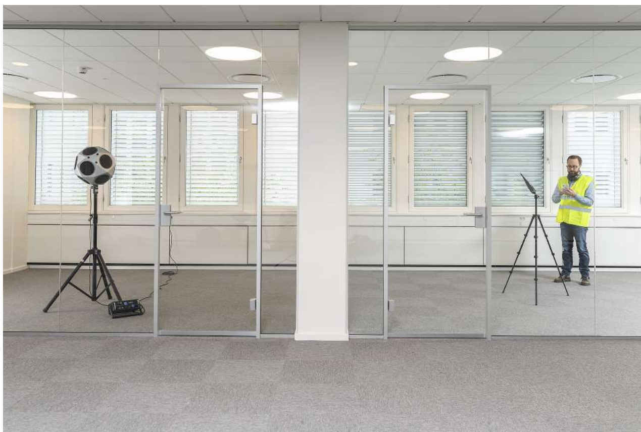
Figure 5: Example of measurement, the HBK 2255 sound level meter and HBK 2755 amplifier can be operated (wirelessly) via smartphone .
